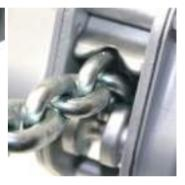
The fluted chain stripper is specifically designed to guide the load chain safely onto or off the load sheave. The critical configuration of, and distance between, the chain stripper and the roller guide ensures alignment of the chain so it cannot snag or jam. This allows the safe use of the SS19/PROLH when used in any orientation.
