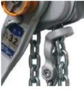
Tiger have incorporated the ultimate safeguarding of a single point failure mode as described in IMCA DO28 Rev. 2 Note 7.2 by installing a specially designed adjustable chain end stop. Tiger have specifically profiled and manufactured this item to fit the contours of the SS hoist. This offers complete assurance to the operator, whilst maintaining the flexibility of "freewheeling" the chain to any required starting position
