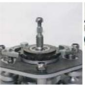
8 point multi-start thread pinion shaft on all our lever hoists and chain blocks- doubles the lead distance compared with typical 4 point threaded shafts, increasing the brake efficiency by 100%.
