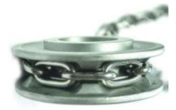
For chain blocks to be used up to an angle of 45 degrees, it's critical that the hand chain leaves and enters the hand wheel without twisting, snagging or jamming. Thanks to our specially designed deep-profile chain block hand wheel this is achievable as it helps to seat the chain no matter what angle or direction of pull.
